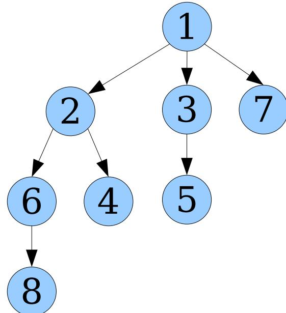
Make the binomial tree with the larger root the first child of the tree with the smaller root.
